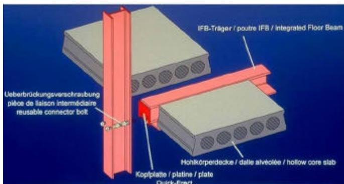
Figure 4. Typical detail of an IFB-slimfloor
